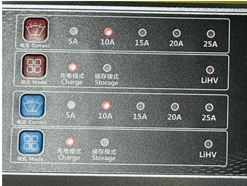
Figure 8: Selecting the battery type and charging rate
