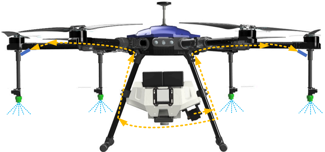
Figure 2: working schematic of spraying system
