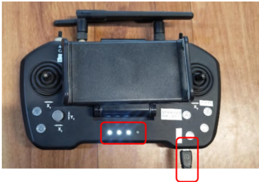
Figure 40: Charging port on RC
