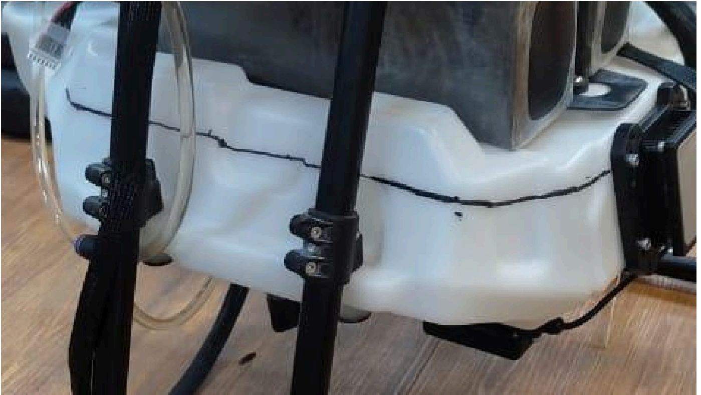
Figure 9: Maximum Tank Filling Marking on Tank
