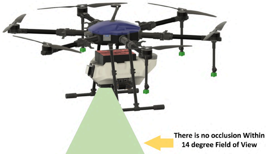
Figure 8: Terrain following sensor working schematic
