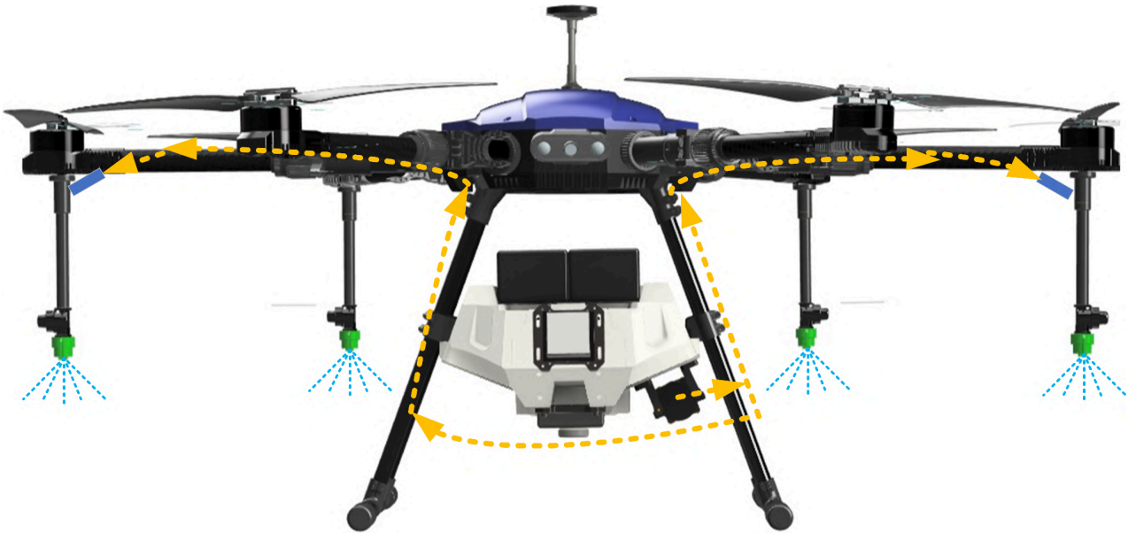
Figure 12: Physical working of spraying system
